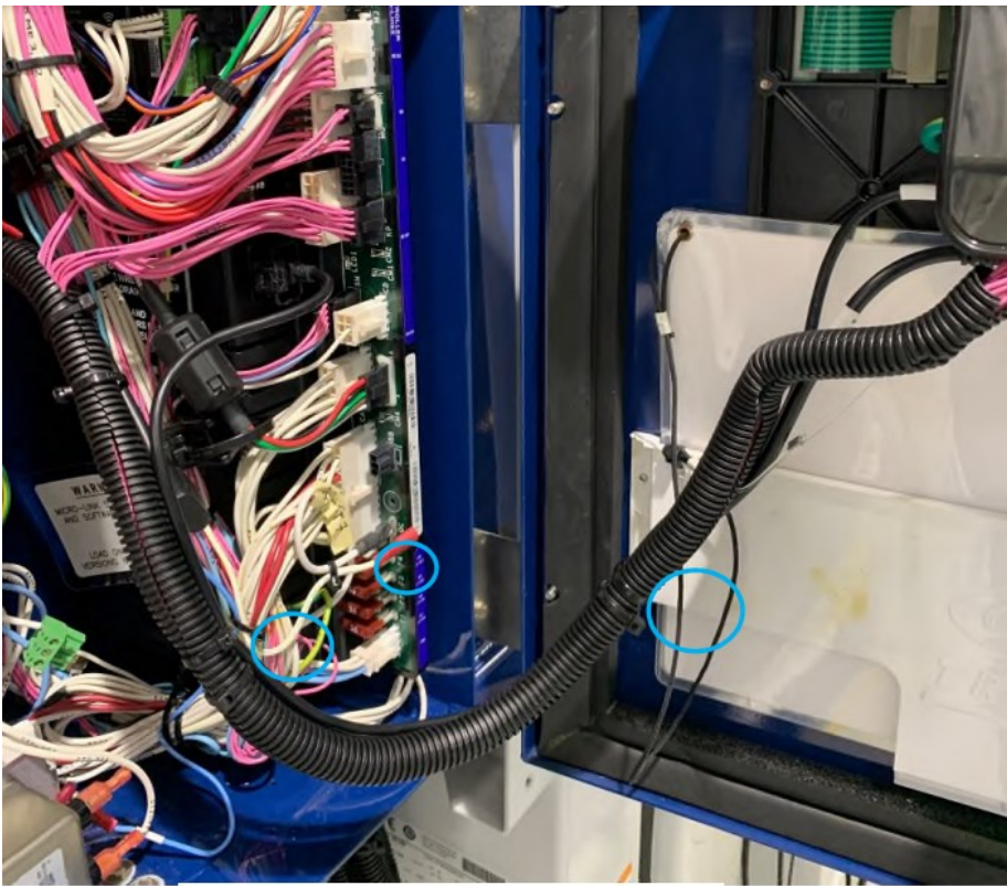
Figure 7a: Securing wire harness
