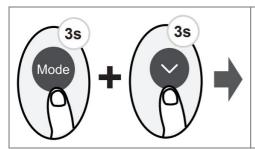
Press together Mode button and "\" button at the same time more th an 3 seconds to activate this function, and the remote controller displays "F2". When setting the panel status, press the "\" or "\" but tons of the remote controller to control the rise or fall of the grille, and p ress any other button to exit the setting.
