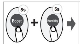
Press together Boost button and Humidity button at the same time mor e than 5 seconds to activate Lock function.
