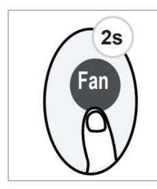
Keep pressing Fan button for more than 2 seconds to activate/disable Silence function(some units).
