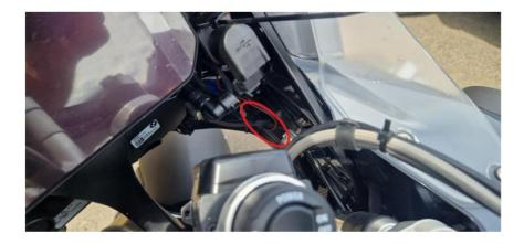
On older models the connector is located at the front under the motorcycle dashboard.
