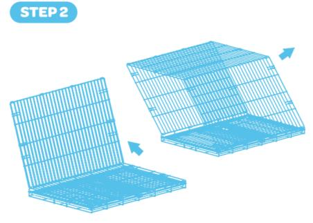
3. Hold the top panel up, reach inside the crate and pull the door panel forward until it snaps into the 7 hooks located around the edges of the crate.
