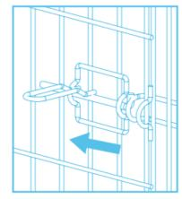
2. To close, lift up and slide the locking handle to the left and shut the door. Slide the locking handle to the right and push down to secure the locking handle to the crate frame. If your crate has more than one locking handle repeat step for all locking handles to open the door.
