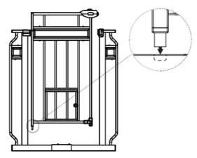
3. Align the hole in the upper corner of the gate door with the hole in the door mounting bracket. Insert the spring-loaded mounting pin (I) into the hole in the mounting bracket and the door.
