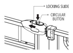
**NOTE:** If your secure slide latch is not properly engaging with the receiving component, ensure that your gate is level, mounted properly, and that you have not over-tightened the threaded spindle rods.
