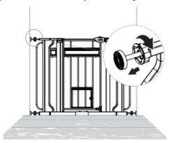
**NOTE:** The gap between the gate and wall should not exceed more than 2.5 inches. Make the appropriate adjustment to ensure you have installed your gate safely.
