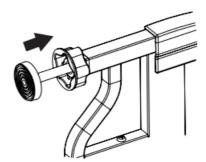
**NOTE:** Once the spring loaded mounting pin is inserted into the gate door hole, it cannot be taken out again by hand.
