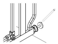
2. With gate fully removed, you can now use the circles you marked during Step 1 as guides for screwing in your (4) wall cups (G). Center each of the wall cups within the guide circles and use the provided self-tapping screws (H) to fasten them in place via the hole through the center of each wall cup.
