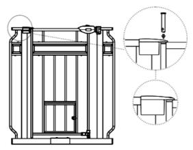
4. Locate the (4) threaded spindle rods (F). Rotate the adjustment wheels along the threading, eliminating the gap between the adjustment wheel and the rubber foot.
