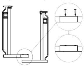
2. Lower the gate door (C) into the assembled gate frame and insert the lower gate door pin into the mounting hole on the frame.
