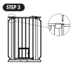
4. Locate the 1:411 threaded spindled: f, E). Rotate the adjustment wheel: along with the threading, eliminating the gap between the adjustment wheel and the rubber foot.
