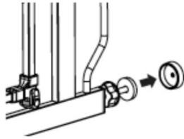
3. Reinstall your gate in the doorway or opening according to the instructions, using the newly installed wall cup: a: anchoring point for the (4) threaded spindle rods.
