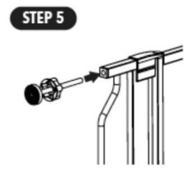
**NOTE:** Once the spring-loaded mounting pin is inserted into the gate door bole, it cannot be taken out again by hand.
