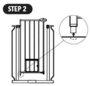
3. Align the hole in the upper corner of the gate door with the hole in the door mounting bracket. Insert the spring-loaded mounting pin (H) into the hole in the mounting bracket and the door.
