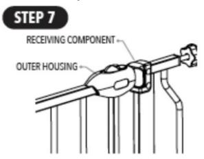
**NOTE**: There should be equal spacing among each of the (4) threaded spindle rods. Make the appropriate adjustment to ensure you have installed your gate safely.
