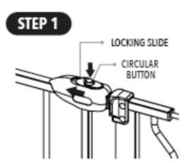
Push the circular button on the secure: lice latch while simultaneously pulling back. These two actions combined will disengage the lock and Tikrit the gate to open the tree). Push or pull to open the gate door. To dose, simply or pull the door bad into t original position. The secure slide latch will re-engage automatically and lock the door into its closed position.
