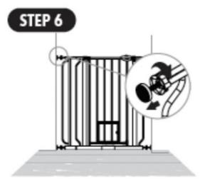
**NOTE:** The gap between the gate and wall should not exceed more than 2.5 niches:. Make the appropriate aal current to ensure you haw installed your gate safely.
