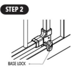
2. At the bottom of the gate door, rotate the case lock to the horizontal potion. To allow the door to swing open in only one direction rotate the base lock on one side. To allows the door to wing open in both directions, rotate the base lock on both sides.
