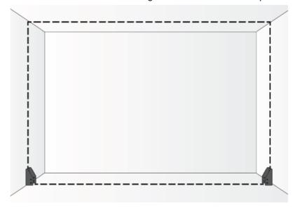
• Then continue with the 2 ceiling corner cable anchors. Install each into the top plate in the same manner, with the tapered end pointing down.
