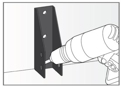
The corner cable anchor is designed to secure the screen with a single screw through the angled hole (as shown). The two holes above can provide additional security. However, they are optional.
