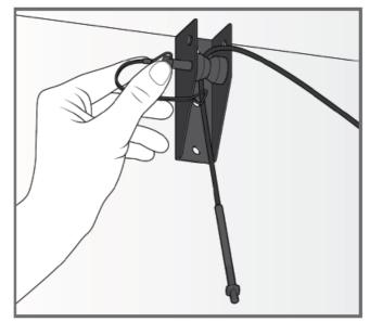
• Repeat with the other ceiling cable anchor. Once secure, the top cable should be spanning the ceiling, with the left and right sides hanging down.
