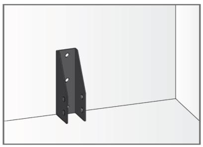
• Make sure the corner cable anchor is level. Then mark the bottom-angled hole and drill a pilot hole at a downward angle for the 1/4" lag screw. Use one screw to secure it in place through the bottom angled hole into the bottom plate of the wall.
