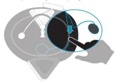
4. Attach the Velcro Pads to the helmet's inner padding
