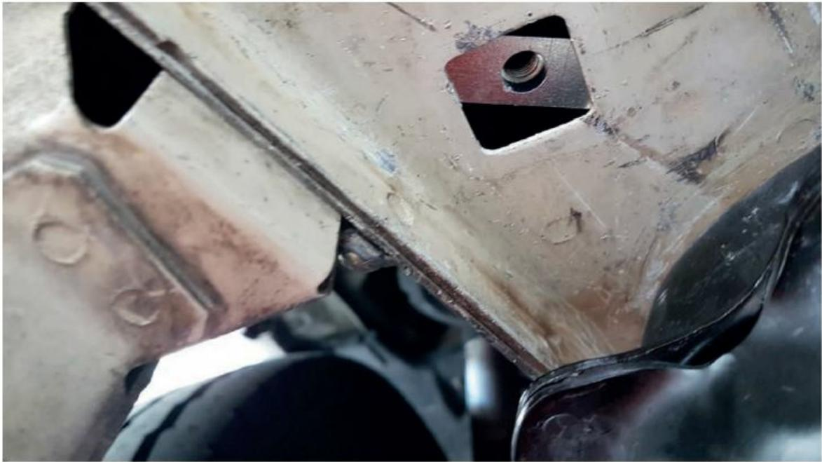
Insert the sealing plate with the screw hole concentric to the square hole in the chassis.
