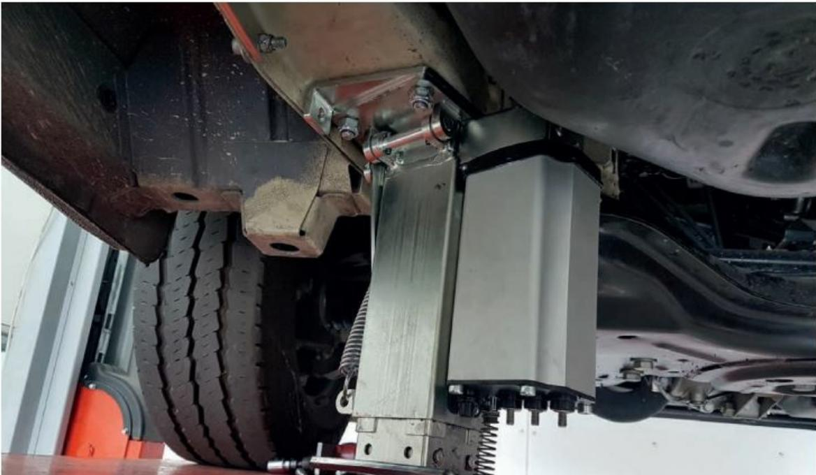
If necessary, loosen the bolts supporting the tank and move it a few centimeter toward the center of the vehicle.
