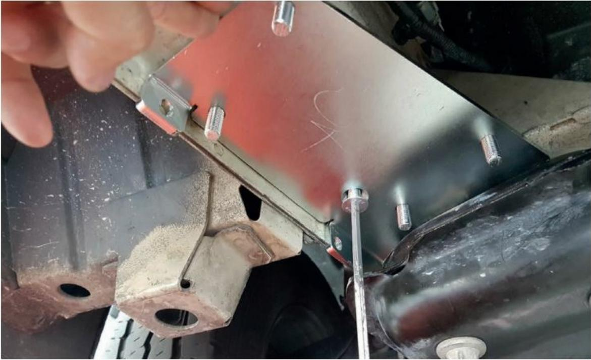
Fix the adapter with the sealing plate that you inserted into the hole.
