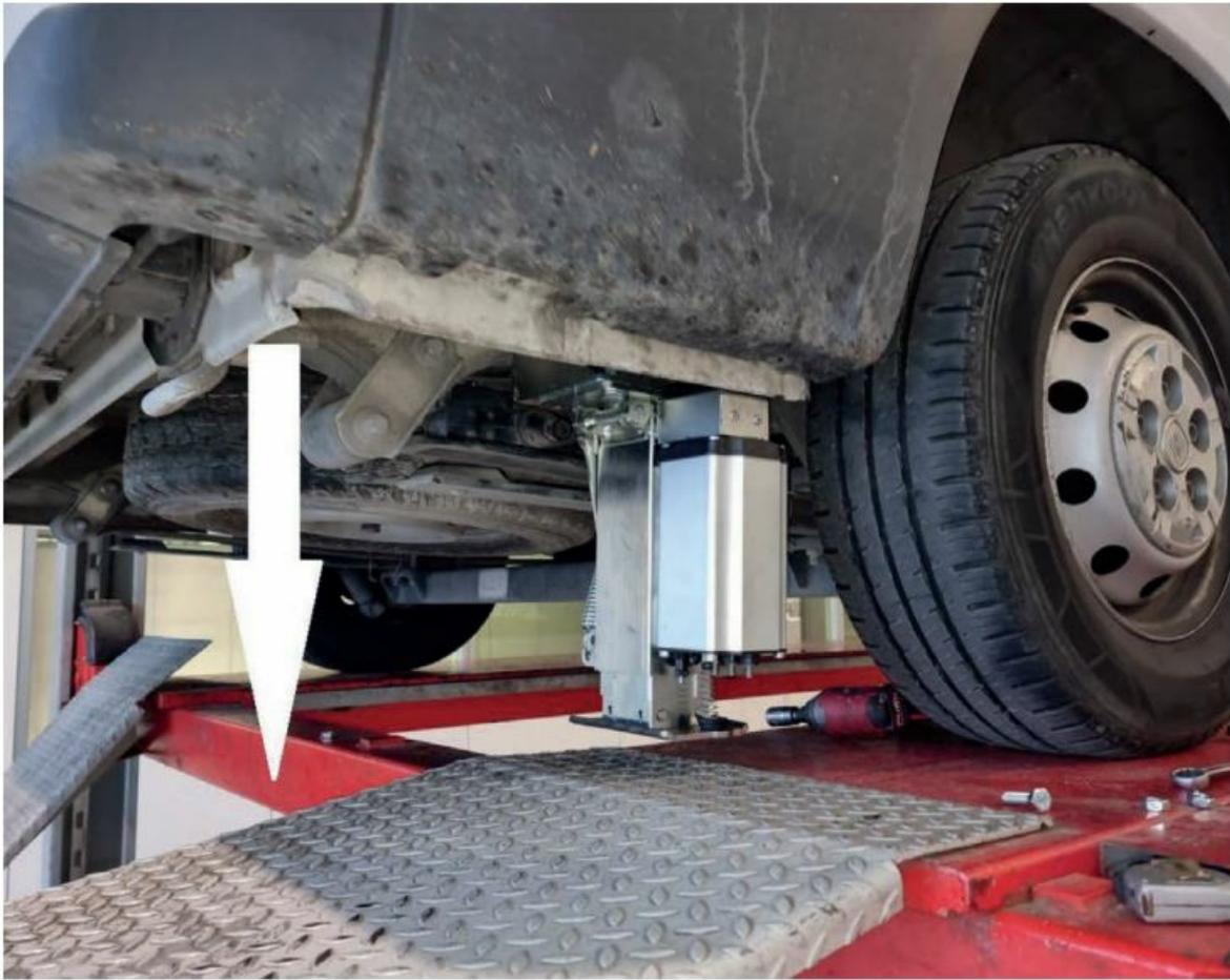
41 CENTIMETER FROM THE TOWING EYE WELDING SPOT TO THE GROUND IN THE POINT INDICATED.
