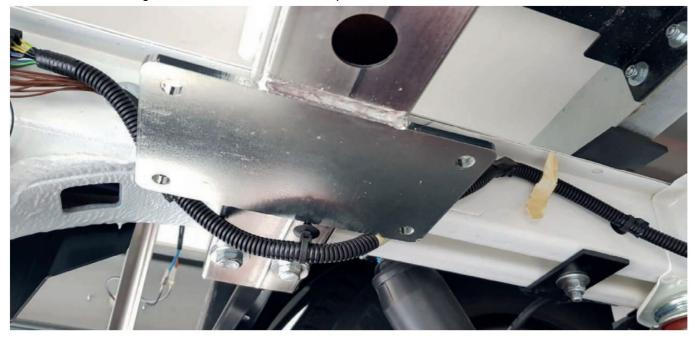
STEP 4: Fix the adapter using 4 10 x 70 mm bolts, then fix the jacks.
