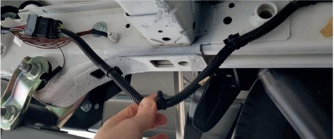
Move the electric wiring to the side, then insert the adapter.
