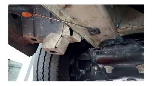
**STEP 2:** Insert the mounting plate into the square hole.
