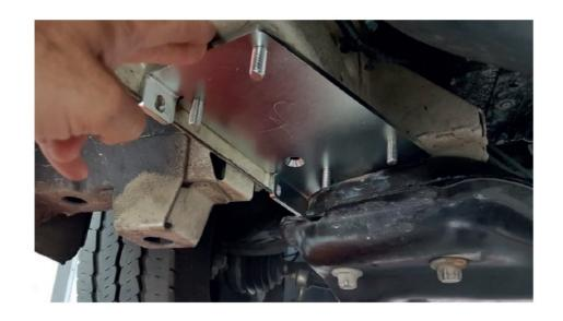
**STEP 5:** Fix the adapter with the mounting plate that you inserted into the hole.
