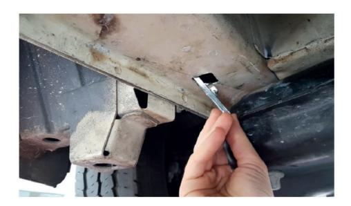
**STEP 3:** Insert the mounting plate with the screw hole concentric to the square hole in the chassis.
