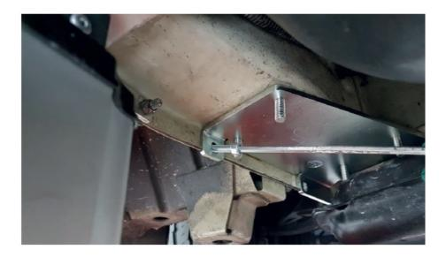
**STEP 8:** If necessary, loosen the bolts supporting the tank and move it a few centimeter toward the center of the vehicle.
