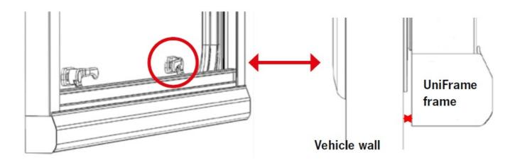
If necessary, insert the spacer profiles into the slot to adjust the height according to the length. Start with the aluminum profiles and then insert the plastic parts.
