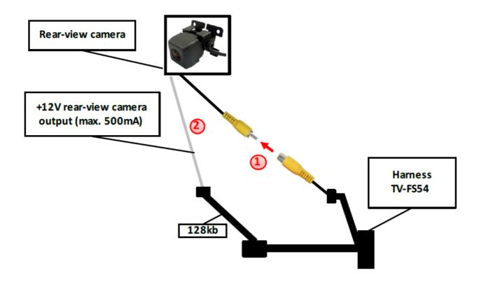
Connect the video RCA of the rear-view camera to the female RCA connector (RVC input) of the TV-FS54 harness. 2. Connect the white cable from the 125kb 8-Pin connector of harness TV-FS54 to the camera power supply (+12V, max 500mA). The white cable gets power when the reverse gear is engaged. By leaving the rear camera level the power is switched off again
