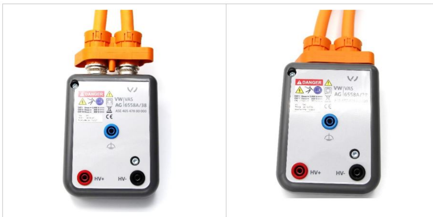
Fig. 3: Insertion position of the high-voltage cables
