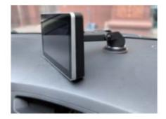
When mounting on the dashboard, you may find the surface of the dashboard is uneven. If so, use the supplied 3M adhesive disk.
