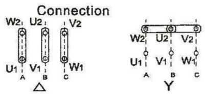
When the power phase ABC are corresponding with the binding post U1, V1, W1, you will notice that the rotation of the motor is clock wise rotation from the main shaft end. If you change the power source phase sequence the rotation direction of the motor will be totally opposite.
