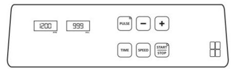
When the instrument is under operation, to change the time value, press TIME button followed by"+" and"-" key to set the desired Time
