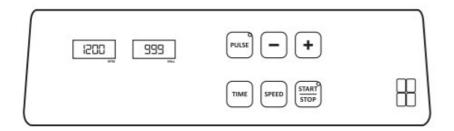
In order to fast forward the increment OR decrement of the speed setting, press + or - button continuously. (for eg: the increment will jump from 20, 40, 60  $\dots$ , as long as we continue to press the + or - button.) The value in the display window will blink 5 times and then stop, confirming that the set RPM value has been saved.
