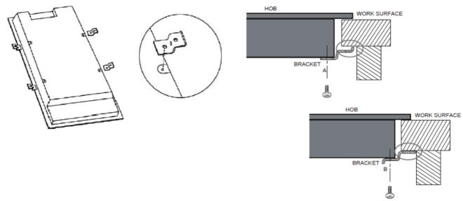
• Under any circumstances, the brackets cannot touch with the inner surfaces of the worktop after installation (see picture). This will ensure the hob is properly secured to the underside of the work surface.
