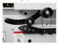
• Overam blade guard with quick change straigth and bevel guards
