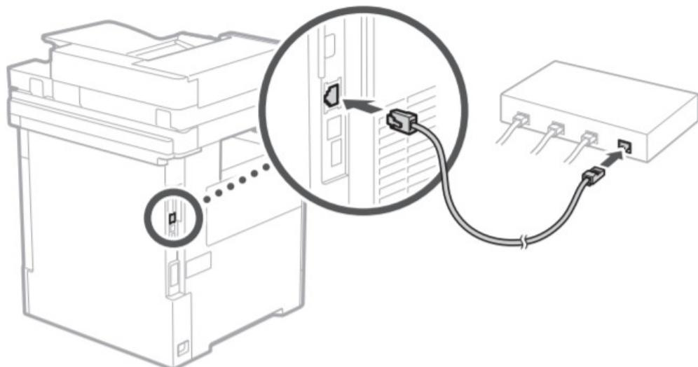
2. To use the machine for faxes, connect it to the phone line using a modular cable.
