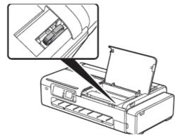
• Check that the roll holder and roll holder support are removed.
