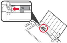
3. a Load plain LTR or A4 size paper against the right edge with the print side facing up. b Slide the paper guide to align it with the side of the paper stack.
