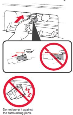
4. Push the FINE Cartridge in and up firmly until it snaps into place.
