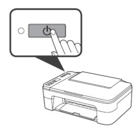
If E > 0 > 9 appears on the screen, press the ON button to turn off the printer, and then redo from step 2.
