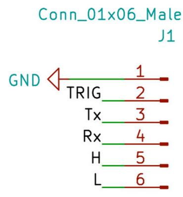
The **TRIG** pin is controlled from GPIO2 on the Pico. This can be driven by software to trigger a test instrument when certain conditions are observed. It can also be used as a general-purpose debugging pin (e.g. for measuring the execution time of sections code).
