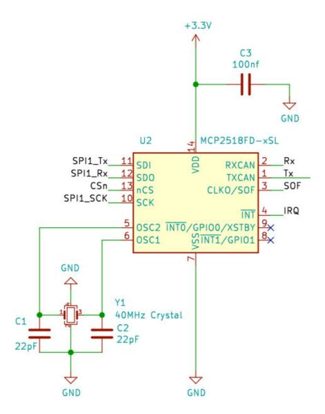
The CAN controller is clocked by a 40MHz crystal and the SPI clock from the RP2040 on the Pico can go up to 18.5MHz. More details on the SPI interface can e found in section 4 of the CAN controller datasheet (available from Microchip).
