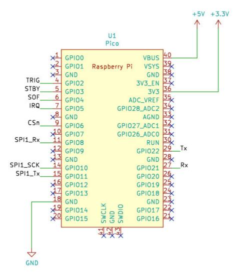
The Pico should be soldered to the CANPico at the 13 pins shown in the schematic above. The Pico has castellated ("half-moon") edges to support this, allowing
