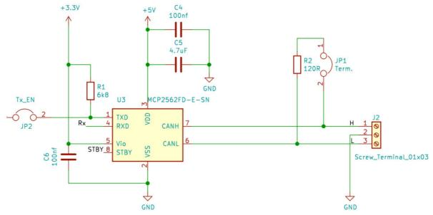
The TXD input to the transceiver comes from either the CAN controller or a GPIO pin from the Pico (the latter is to allow the software to emulate aspects of the CAN protocol). The signal goes through jumper JP2 ("Tx\_EN"): if this is not closed then a pull-up resistor holds TXD high and no software can send signals on the CAN bus (this is useful if the software on the Pico is to monitor a CAN bus without the possibility of disturbing it).
