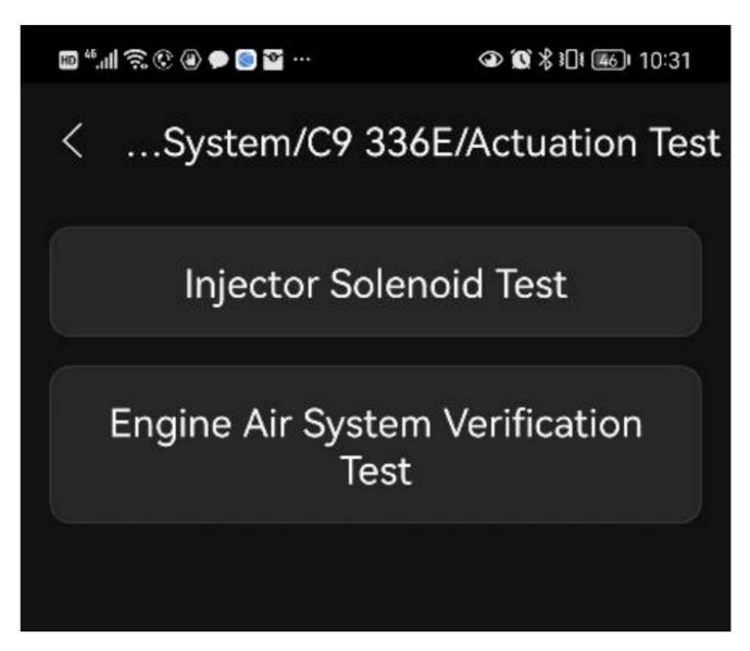
• **Special Function:** By executing this function, you can do self-adapting for each component. It is mainly used to re-calibrate or configure the components after repairing or replacing components, so that the components of the electronic control system can adapt to each other, otherwise the system will not operate normally.
