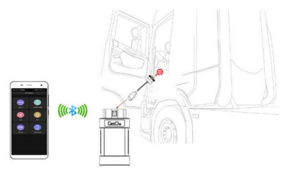
**Note:** at this time, the device is powered by the vehicle diagnosis seat, and the device starts automatically. If not, it may be that the vehicle diagnosis seat has no power supply, and the equipment can be powered by the cigarette lighter or battery clip.
