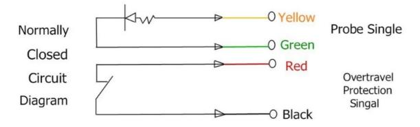
**NOTE:** the wire colors may vary between vendors on these unit. Get the diagram for your model . The ProbeSingle needs a voltage source . While it reports to be a NC (norally cloased ) device its been or experinece the button sensor is NO while the overrun is NC.
