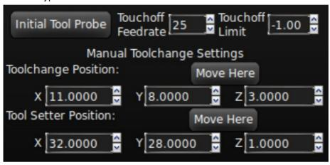
The Touch-off Feedrate sets the speed at which the tool will move down to the tool setter. This should be fairly slow (10 to 30 IPM) so the tool setter and tool are not damaged.
