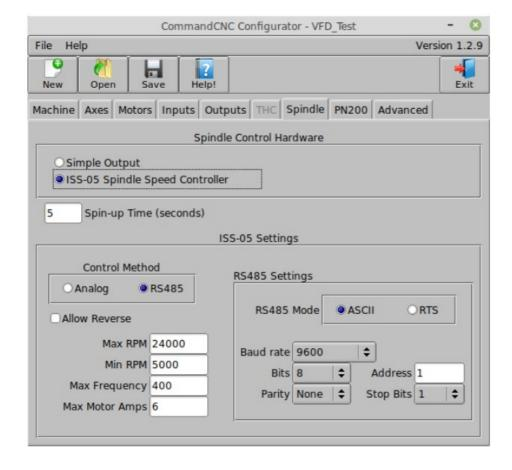
The settings on the left must be set according to the specifications of the spindle motor. This information is usually on a data plate on the motor or in the motor's manual.
