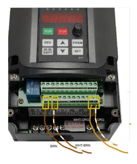
NOTE RS- and RS+ need to be reversed at the VFD . Solid wire goes to RS- , Striped wire to RS+
