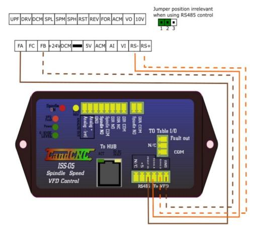
NOTE RS- and RS+ need to be reversed at the VFD . Solid wire goes to RS- , Striped wire to RS+ +
