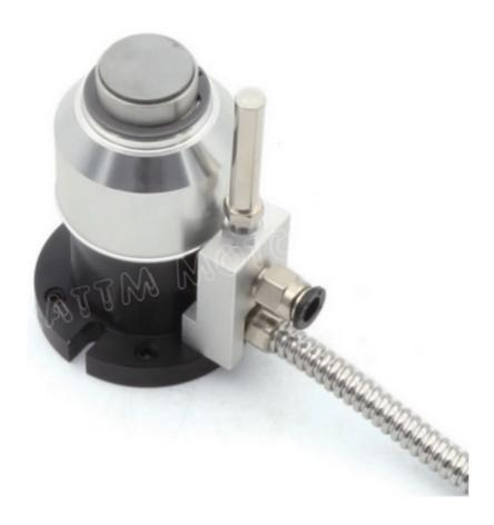
The strange looking tube on the side is not some electronic sensor. Its an air tube that connects to the air input down by the cable and keeps cips off the topof the sensor button. The one shown goes for 50 to 7 bucks from China if you don't mind waiting 4 to 6 weeks to get it, We have tried several and the do the job and they have the overrun sensor built in . They are rather tall at well over 2 inches so you have to be mindful of the Z height to rapid over to he tool setter device
