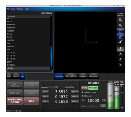
The spindle section of the CommandCNC screen will only appear if the ISS 05 is selected in the Configurator. It has buttons to start and stop the spindle as well as set speed for manual work. There are +/- buttons beside the spindle speed DRO which can increase or decrease the speed in 100 RPM increments. This works even while running gcode. The slider below that is a spindle speed override which will increase or decrease the speed as a
