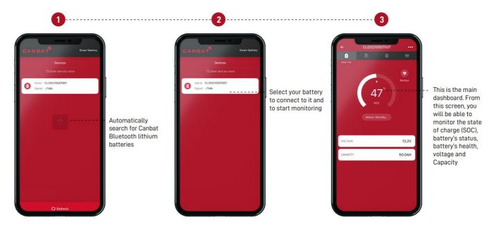
If you search and do not find your Canbat Bluetooth lithium battery in the search results, it may be because another device is already connected to it. Only one device can be connected at a time. For example, you can either connect the battery to your smartphone or your tablet, but not both simultaneously. This applies to IOS & Android.
