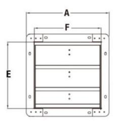
Canarm's GSF series wall exhaust fans are ideal for light commercial applications. The fans have a galvanized frame with aluminum shutters.
