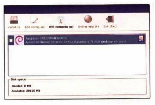
**NOTE:** If the device stops at the rainbow splash screen as shown to the right, or there is nothing displayed, ensure you are using Raspberry Pi 4 compatible software such as NOOBS 3.1.0 or later. Refer to the troubleshooting section on.
