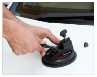
• Now loosen the knob on the suction cup, then attach 110mm rod to it and retighten with the same knob.
