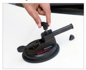
• Loosen the knob from joint clamp and attach it to 110mm rod.
