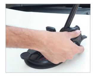
• Attach the joint clamp to the camera platform. Using the same approach, attach other joint clamps to the camera platform and tighten the knobs. Then attach 450mm rod setups to it.
