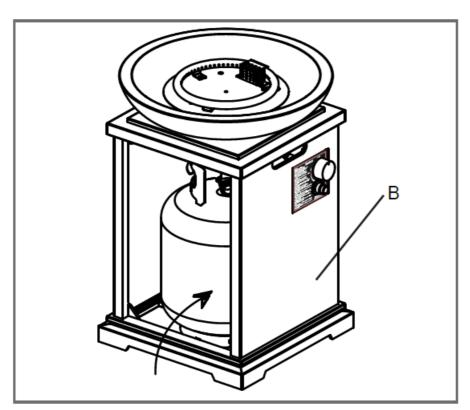
3. Turn the cylinder valve on the tank clockwise to close the propane tank. Attach the preassembled regulator from the body to the cylinder valve by turning the regulator coupling nut clockwise. Make sure it is fastened securely and tighten connections by hand only.
