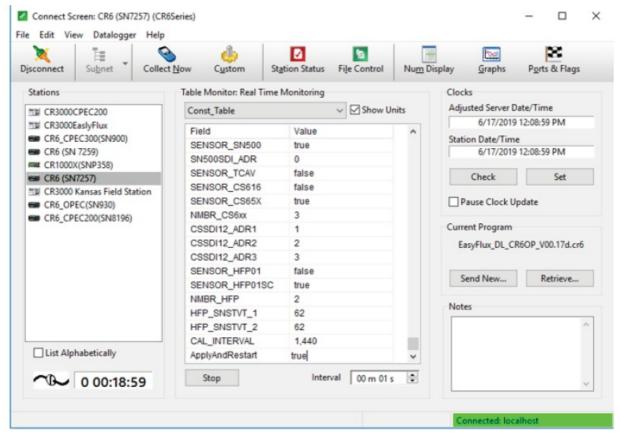
4. Once all of the sensors and constant settings are correct, scroll to the bottom and set Apply And Restart to true.
