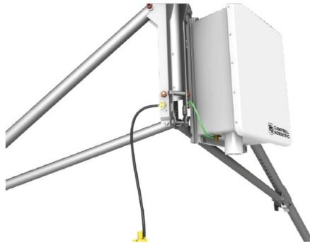
3. Attach the CM20X crossarm to the tripod mast.
