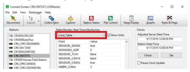
3. Set all the sensors that are used in the system to TRUE and declare their address, quantity, and calibration information. Select the cell to be changed, right-click on the cell, then select View/Modify Value to change the setting.
