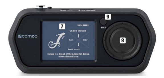
The UNICON remote unit has both a touch display and a rotary-push encoder with an additional BACK key. Both operating elements provide full access to all unit options.
