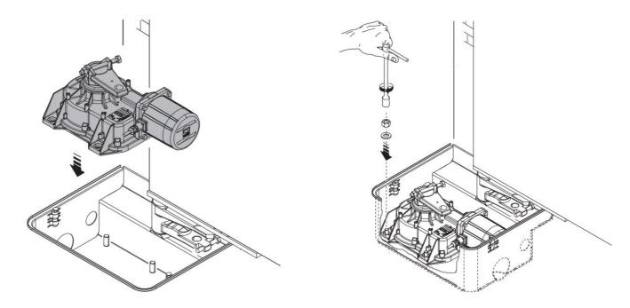
Lubricate the transmission lever. Fit the transmission lever as shown in the drawings.
