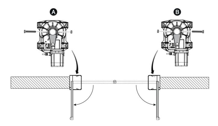
Manually open the leaf. Position the gearmotor over the threaded pins of the casing and fasten it.
