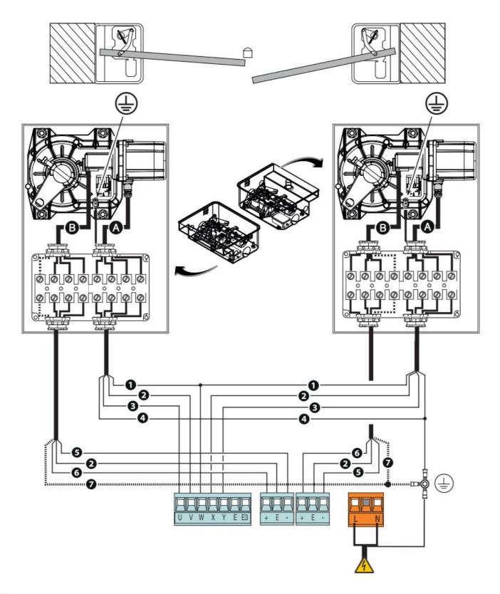
Check the correct direction of rotation of the gearmotor and, if necessary, invert the connection of the brown and black cables.
