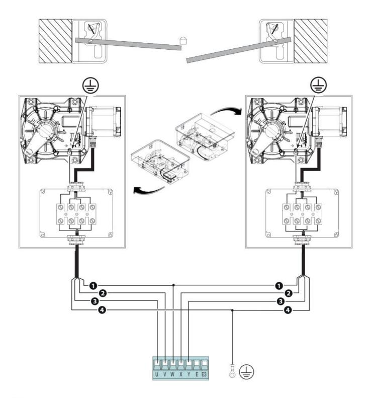
Check the correct direction of rotation of the gearmotor and, if necessary, invert the connection of the brown and black cables.
