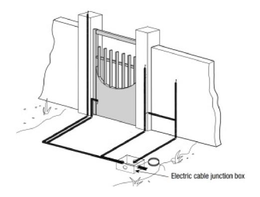
1. Trace the center lines and external dimensions of the entire assembly in accordance with the diagrams on pages 2 and 3.
