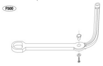
**2b)** Secure the runner to the wing and insert the straight arm.
