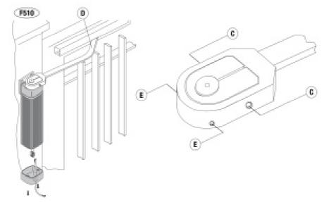
6. Complete installation by mounting the upper cover with its OR gasket.
