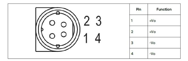
• -V is connected to AC input ground.
