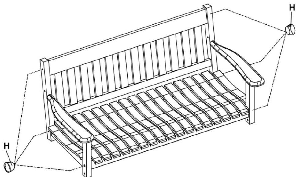
Tighten all bolts completely using a screwdriver and tipping in the wooden caps (H). to cover bolts-head using a rubber mallet.
