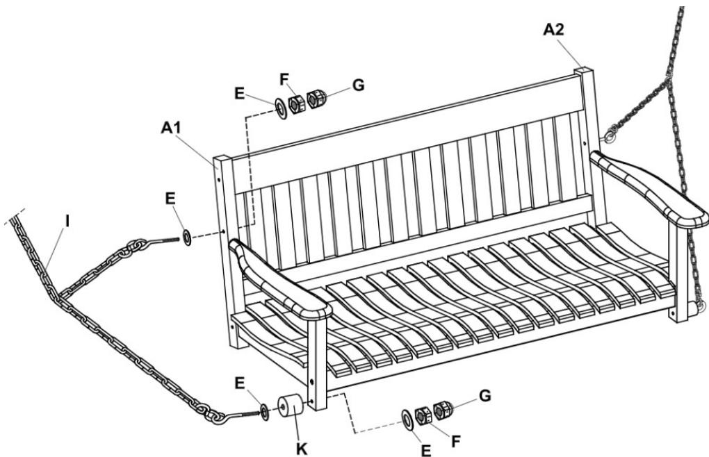
Secure the hanger bolts with chain (1) into predrilled holes of right side frame (A1), using washers (E), dowel rings (K), nuts (F), and head nuts (G) as shown. (The hanger bolt with a long chain must be installed in front). Repeat the same procedure to install the hanger bolts (1) into the left side frame (A2). Make sure all parts are correctly connected and tighten all nuts completely using a wrench.
