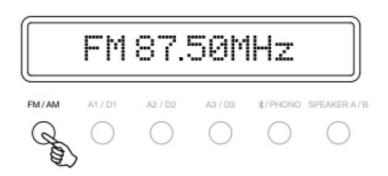
Repeatedly pressing the FM/AM button on the front of the unit switches between FM and AM modes. **Note:** For ease of tuning on first-time use, we recommend that you set the AXR to 'Auto' mode. Press the Mode/Store button on the front of the unit.
