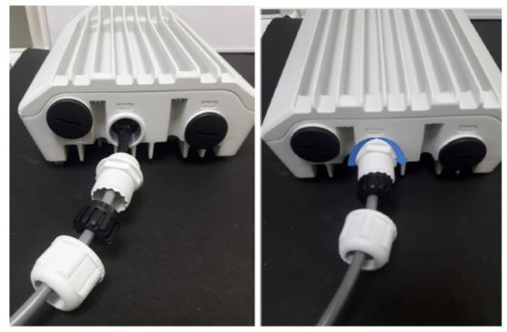
4. Rotate the gland clock wise to tightly fit the gland on the PSU port.
