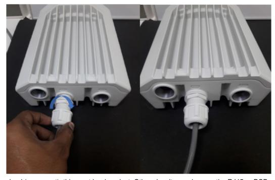
5. Tighten the gland (cap or nut), this must be done last. Otherwise, it may damage the RJ45 or PCB.
