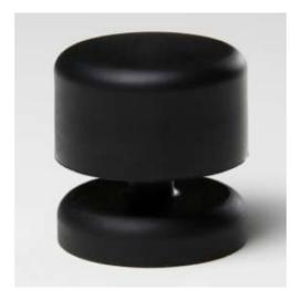
Congratulations, you are the owner of a brand-new ULTRASONIC Wind Instrument and Data Logger. A wireless (BLE) and battery-powered pocket-sized ultrasonic anemometer, is easy to install, simple to use and compatible with IOS, Android and Garmin watches.
