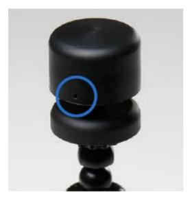
The Ultrasonic Portable Mini has to be oriented to the bow taking as reference the mark that appears on the side (as shown in the image below).
