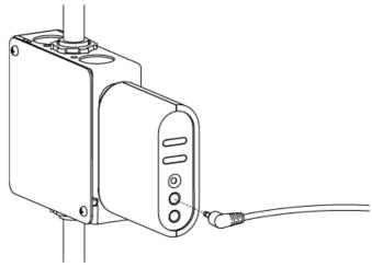
2. Plug the probe into the controller's temperature port.
