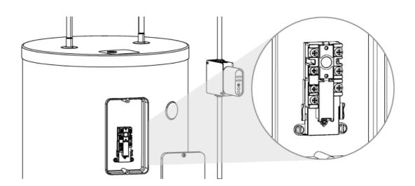
1. Unscrew and remove the door plate located at the top of the water heater.
