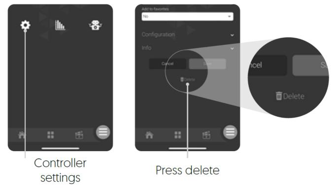
• To remove your controller from Neviweb, press Delete in the controller settings.
