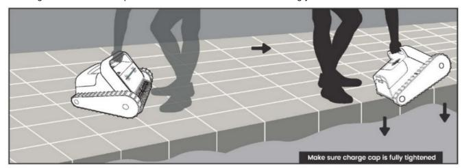
2. Hold the cleaner in water for a few seconds as it releases air trapped in it. Keep the cleaner steady and do not tilt.
