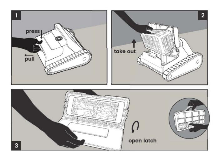
It is highly recommended to clean the filter basket after each cleaning cycle.
