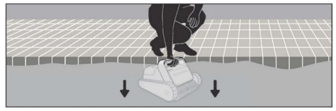
3. Release the cleaner. It takes about 1-2 minutes to complete the self-test and start the cycle.
