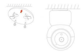
Using the mounting plate the HWC102PT can also be mounted on a wall or ceiling (video image can be adjusted/flipped)
