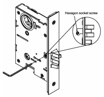
3. Pull out the latchbolt , and turn 180° degree
