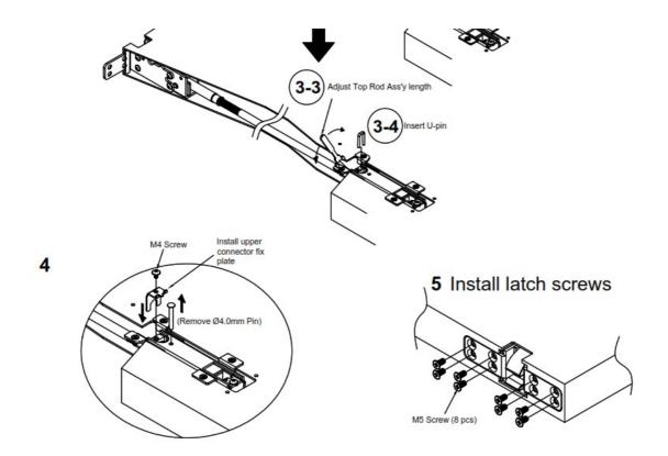
**INSTALL BOTTOM LATCH (Skip this step if less Bottom Rod)**
