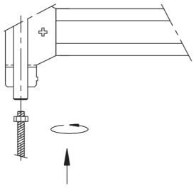
3. Push the top latch in order to turn the threaded rod anticlockwise 15mm to 20mm into the top latch
