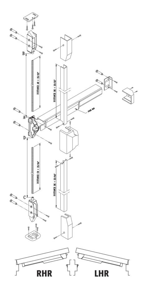
1. Turn the threaded rod clockwise about 15mm to 20mm into the bottom latch
