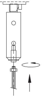
4. Push the bar again and turn the threaded rod into the connection clockwise about 5mm to 10 mm
