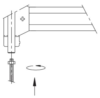
2. Push the bar first and then pull the threaded rod in order to turn it 5mm to 10mm into the connection anticlockwise
