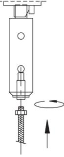
3. Push the top latch in order to turn the threaded rod anticlockwise 1 5 mm to 20mm into the top latch
