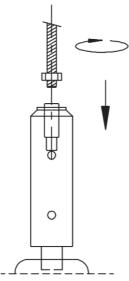
2. Push the bar first and then pull the threaded rod in order to turn it omm to 10mm into the connection anticlockwise
