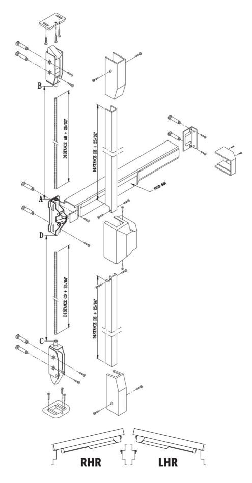
1. Turn the threaded rod clockwise about 15mm to 20mm into the bottom latch
