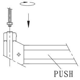
5. Test the movement, and then tighten the nut put on all the other parts.
