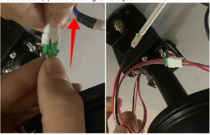
Put the controller on the bracket after all wires well connected
