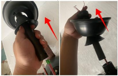
Insert the lever into the motor, then insert the needle/pin, and secured with the screws
