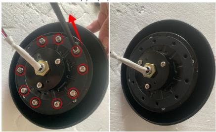
Assemble the blades (4) with the 10 screws to the motor (9)
