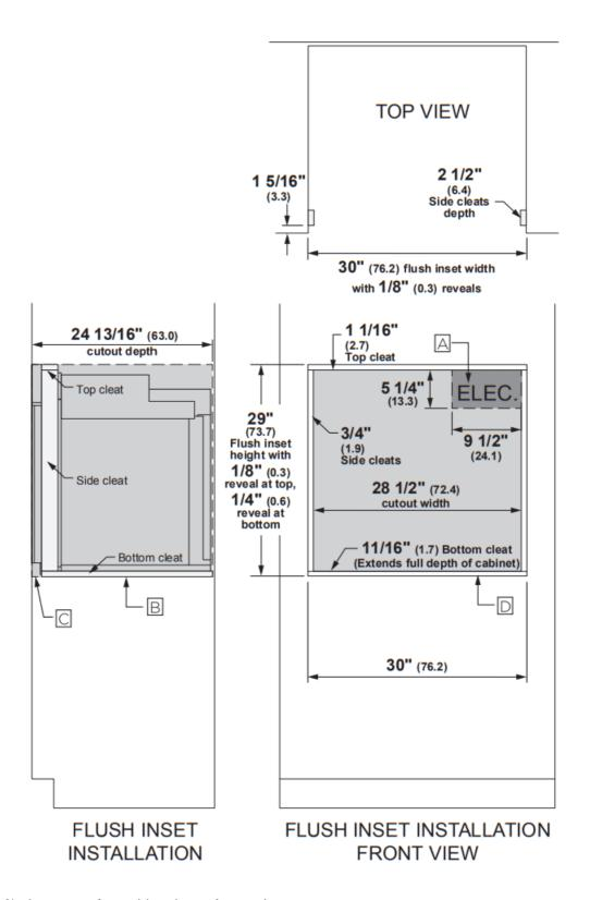
Allow 1/8" (0.3) clearances from side edges of oven door. **Dimension and installation information are shown in inches.**
