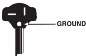
Plug Configuration NEMA #6-20P
