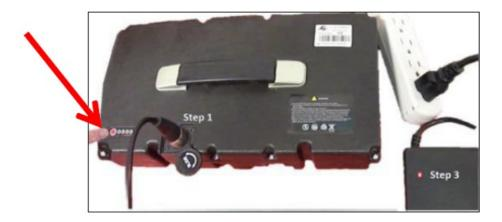
• To check the battery level, press the RED button on top left of the battery (see photo).
