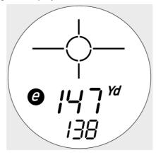
Automatic power-off occurs when the button is not pressed for 10 seconds
